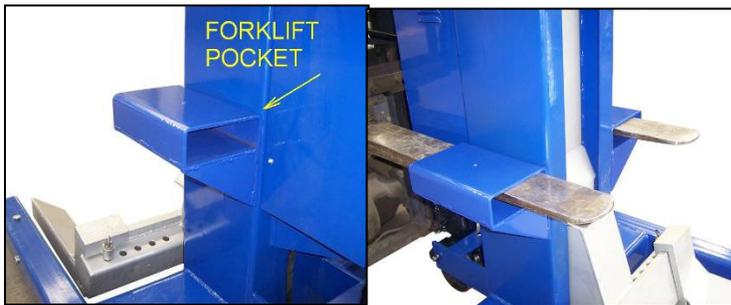
Fig. 3 Forklift Pocket on Column
