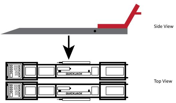
You can put the Lift Adapter Kit onto the QuickJack frames when the QuickJack frames are on the ground or in the first locked position. If you are having trouble putting on the platform with the QuickJack frames on the ground, try raising the frames to the first locked position. If you do put the platform on with the QuickJack frames in the first locked position, make sure to lower them before trying to put a vehicle on the platform.
