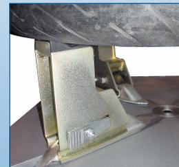
Quickly attaches over clamps to accommodate motorcycle wheels.
