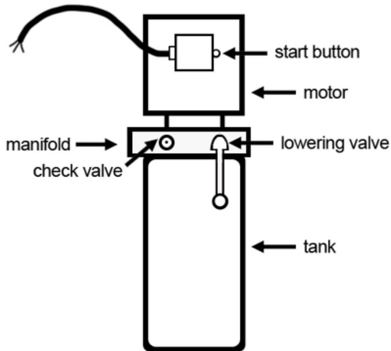
**Step 2** – Using a Hex wrench and shop towel – with shop towel in place to catch fluid – loosen the check valve plug by approximately 2-½ turns and allow fluid to bleed off.
