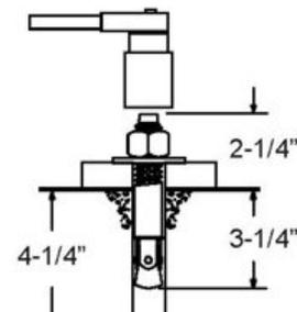
Tighten nut with Torque wrench to 130 ft.-lbs.
